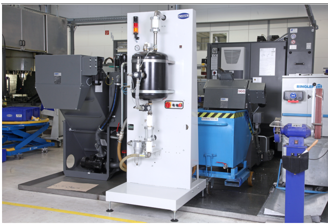
Vacuum Operation Center VOC for vacuum generation in wet working conditions
