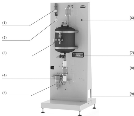
System design Vacuum Operation Center VOC
